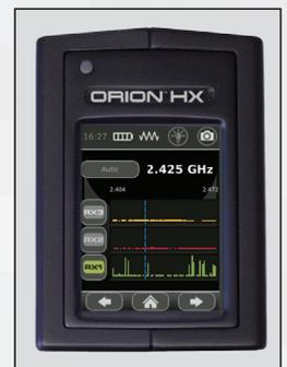
Frequency adjust screen displays Transmit, 2nd, and 3rd frequency ranges.
