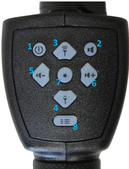
1. **POWER** – Press to Power on. Press and hold while the unit is on to Power off. A tap of the power button while the unit is on allows for quick selection of the Transmit Power Mode (Auto or Manual)
