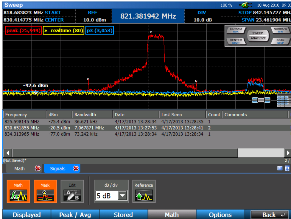
Mask Example: Detecting the presence of a cell phone call
