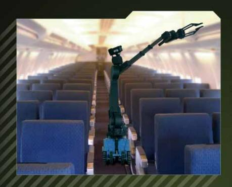
Neutralizing and assisting (EOD/IEDD) Expert robot, as the first one worldwide, may be used for any mission inside means of transportation, e.g.: aircrafts, buses, train coaches, vessels and any other small and tight spaces.
