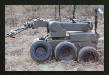
**IBIS** is a robot for pyrotechnic and combat missions. It is designed especially for operations in difficult and diverse terrain (including sand, snow, rocks). High speed of the robot enables taking dynamic actions. Robot's manipulator provide big range of activities and applications. Precision drive system gives fluidity of the movement of every part of the robot, even during fast ride.
