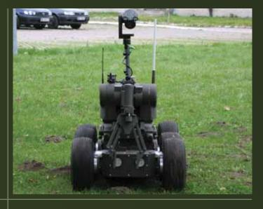
The equipment of the robot can be extended with other devices chosen by the client or developed according to the special order. It is also possible to modify the robot to adapt it to the client's needs.
