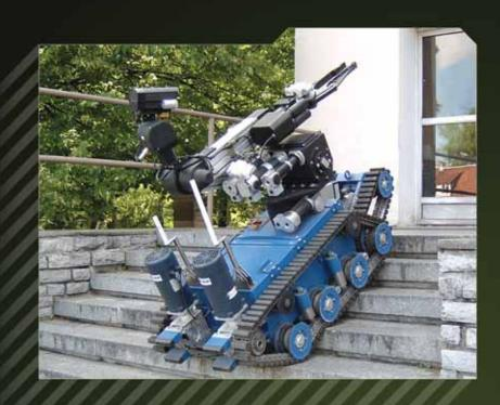
In its class, the inspecting and neutralising (EOD/IEDD) Inspector robot is distinguished by its great lifting capacity and the ability to travel in difficult terrain and to overcome its uneven surface and high obstacles.
